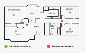
For optimum smoke detection, it is recommended that each smoke alarm is placed on the ceiling, close to the centre of the room, and at least 30cm away from the wall. Keep away from what is known as dead air space where walls and ceilings meet. Smoke alarms may not operate in these areas.
