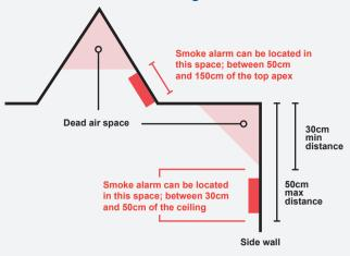
Consideration should also be given to the effect on smoke alarm performance from air conditioners, heaters, fans, air vents and other temperature control devices. Smoke alarms should be located where these devices will not compromise the effectiveness of the smoke alarm.
